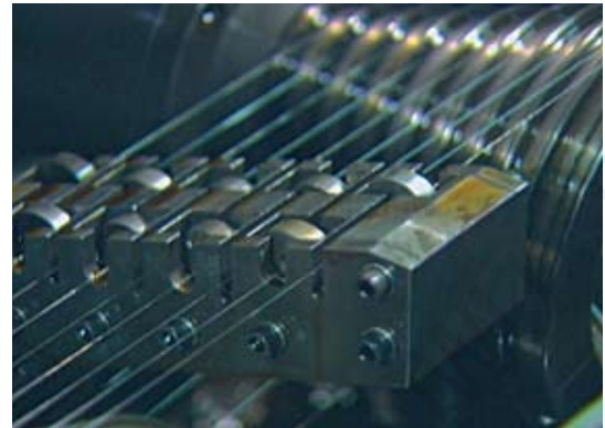
Inside the wire drawing machine
